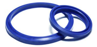
Also known as Scraper Seals or Dust Seals, the primary use of a Wiper seal is to prevent dust, debris and moisture entering the gland housing of the sealing system and damaging the pressure seals of a fluid system as reciprocating or rotating parts move. Without a wiper seal, the retracting piston rod could transport contaminants into the Hydraulic cylinder.
