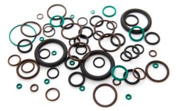
O-Rings are used in automotive applications for sealing a variety of fluids. O-Rings are available in all AS568 inch sizes and a wide range of metric sizes (DIN 3771. ISO 3601 and JIS B2401) as well as custom sizes. O-Rings can be moulded in a wide range of elastomer compounds including PTFE, HNBR and special grades of Viton<sup>®</sup>. HNBR or Viton<sup>®</sup> O-rings are designed to meet the demands of oxygenate-rich gasolines, harsh engine oils and high engine temperatures.
