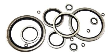
Bonded seals can be utilised for a wide variety of automotive applications including engine sensors, fuel, braking and air conditioning systems. Bonded seals are primarily used in high-pressure environments where copper washers are unsuitable. Both the metal washer and the rubber material can be selected to suit a given application.
