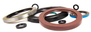
Rotary shaft seals, also known as radial shaft seals or just simply oil seals are used throughout automotive industry in many diverse applications. Rotary Shaft Seals are available in a range of seal geometry configurations and compounds including Nitrile, Viton® and PTFE. They are produced in single or double lip, with covered or uncovered metal parts, with reinforced textile rubber or reinforced metal case, as well as in many other different profiles.
