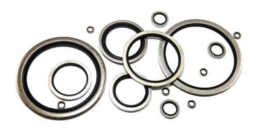
Bonded seals are available in several FDA conforming materials. They can be utilised for a wide variety of applications, although primarily used in high-pressure environments where copper washers are unsuitable. Both the metal washer and the rubber material can be selected to suit a particular application.
