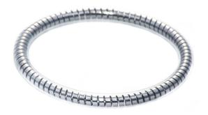
Spring O-rings are ideal for sealing at extremely low temperatures where traditional elastomers suffer from brittleness, and it is very difficult to achieve effective liquid or gas sealing. Low compression sets allow effective sealing as low as -250°C in Cryogenic applications.
