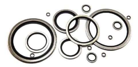
Bonded Seals are also known as Dowty Seals or Dowty Bonded Washers. They are high pressure seals which are used in the Mechanical, Hydraulic and Pneumatic sectors. They comprise of a metal washer and an elastomeric ring which is bonded inside the diameter. The metal washer prevents over-compression and limits deformation of the elastomeric ring.
